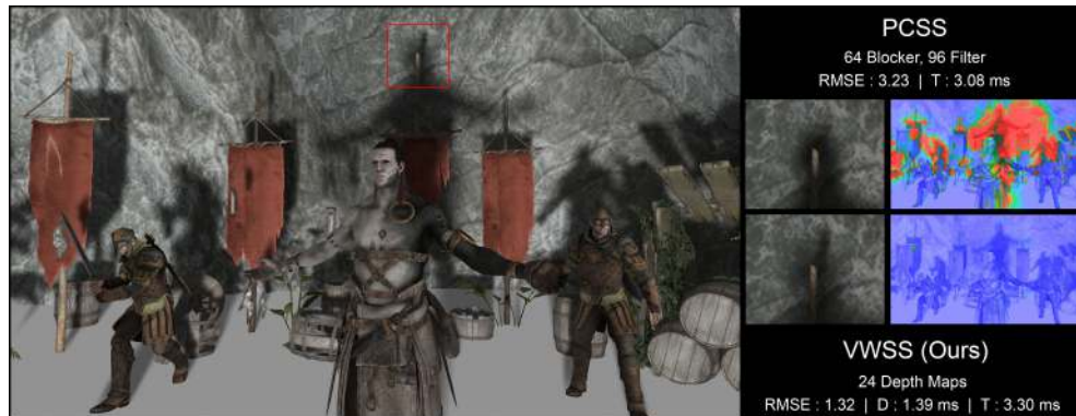
Figure 1. Our method’s soft shadowing of static and dynamic geometry using an area light. The inlays (right) highlight how our approach has soft penumbra and faithfully represents the occlusion relationship of the character’s head and the flagpole. PCSS (percentage closer soft shadows) fails in this situation. HDR-VDP2 heatmaps visualize the perceptual image quality of our algorithm and PCSS compared to a high-quality reference. Blue is high quality and red is low quality.
