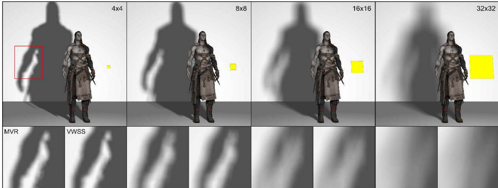
Figure 8. Soft shadowing of the animated Volund character, and a quality comparison of VWSS and MVR as the area light (yellow) grows to 64\times its original area. Additional light samples are distributed across the area light as it grows. A constant rate of one light sample per two units of light area is maintained (ranging from 8 to 512 samples). The value of an algorithm based on reprojection is demonstrated by examining how rapidly the quality of the result declines as the synthesized view(s) diverge from the source view. A close-up comparison (bottom) of shadows generated by MVR (left) and VWSS (right) reveals very similar results even as new light samples are further from the source view located at the center of the area light.
